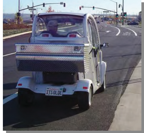
NEV on Class II facility Lincoln, California
