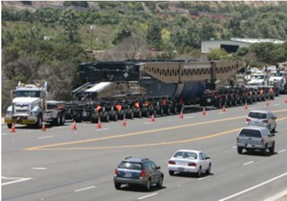
Figure 17-1.1: 700,000 Pound Retired Steam Generator 79
