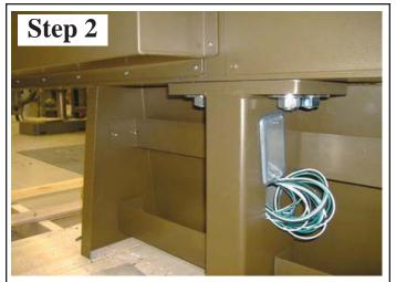
Place front shroud over brackets as shown in photo. Secure with hardware and route wires as needed.
