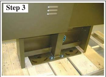
Front shroud shown attached. Place rear shroud on back and secure with hardware.
