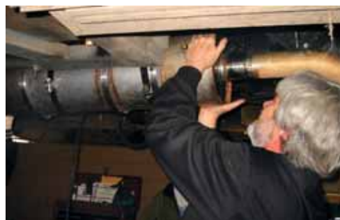
Installing a diesel particulate filter (DPF) in this Atlanta school bus simply required removal and replacement of the muffler and tailpipe.
