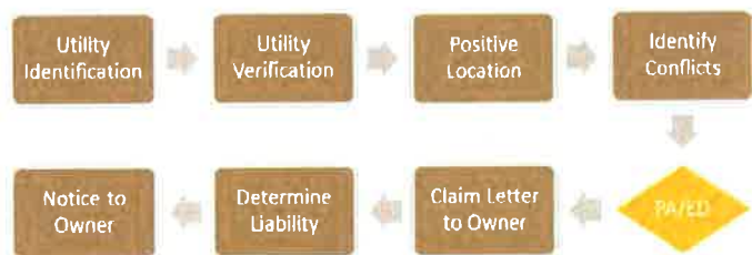
Figure 7 – Accelerated Utility Process
