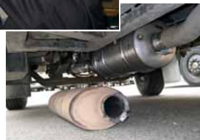
Installing a diesel particulate filter (DPF) in this Atlanta school bus simply required removal and replacement of the muffler and tailpipe.
