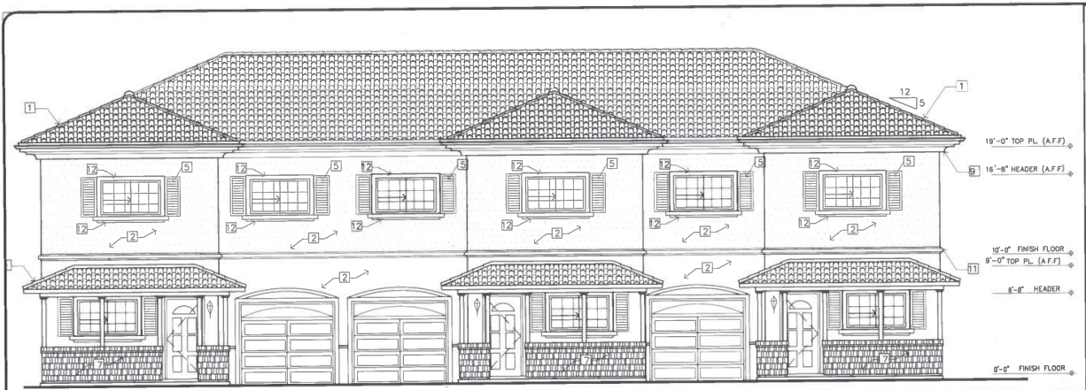
NORTH ELEVATION - BUILDING E SCALE 1/4" = 1'-0"
