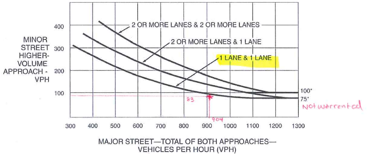
Figure 4C-4. Warrant 3, Peak Hour (70% Factor) (COMMUNITY LESS THAN 10,000 POPULATION OR ABOVE 40 MPH ON MAJOR STREET)
