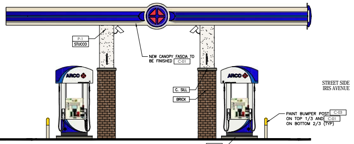
02 CANOPY ELEVATION SCALE: 1/4"=1'-0"
