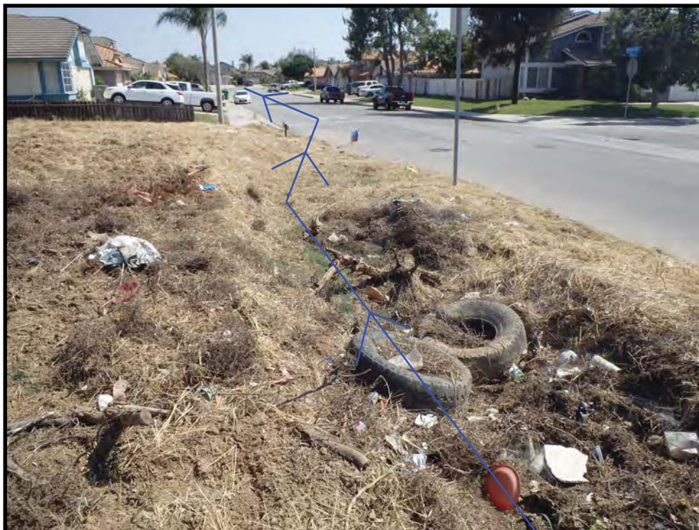
PHOTOGRAPH 4 - Storm water (blue line) flows overland off the Project Site, directly onto Tarano Blvd and then into a storm drain.
