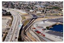
providing a cul-de-sac; replaced the I-110 NB off-ramp with a direct off-ramp to EB Harry Bridges Blvd; widened an existing bridge; and constructed a new bridge. The project also included utilities relocation, fiber optics, signals, street lighting, a new force main sewer valve vault, closing a RR atgrade crossing, and landscaping.
