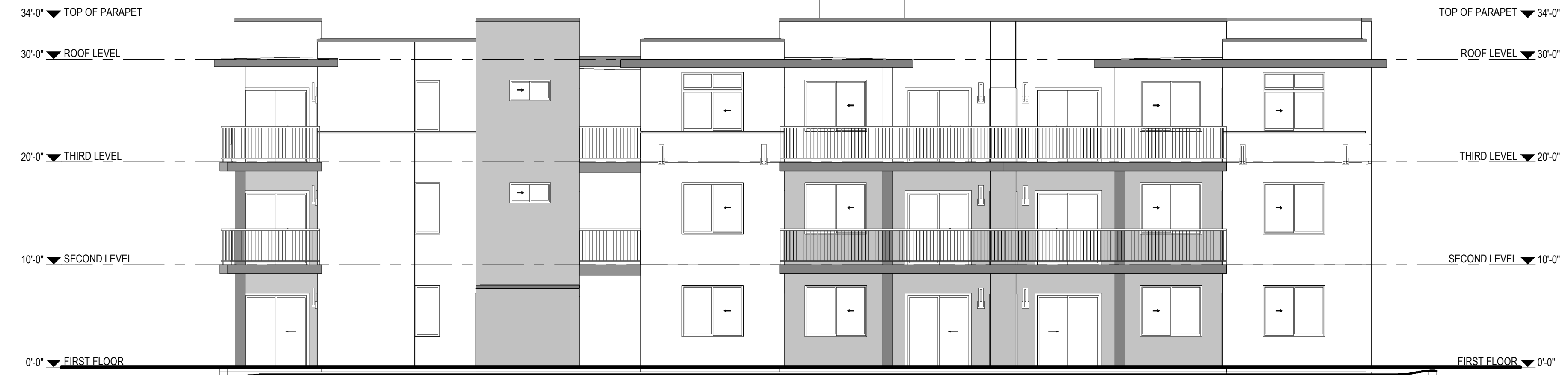
1 APARTMENT BLDG NORTH ELEVATION Ref: A-101 / Scale: 1/8" = 1'-0"
