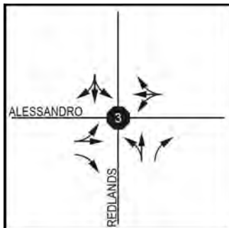
Figure 1 – Existing Lane Configuration
