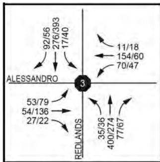
Figure 4 – Existing + Project AM/PM Peak Hour Volumes
