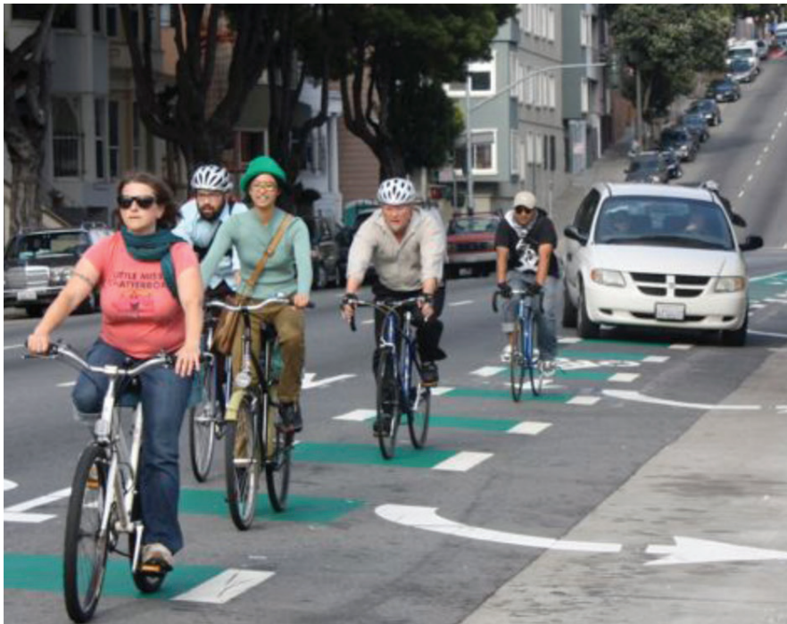
Green transition lanes provide bicyclists a safe crossing through intersections in San Francisco, CA. Source: NACTO
