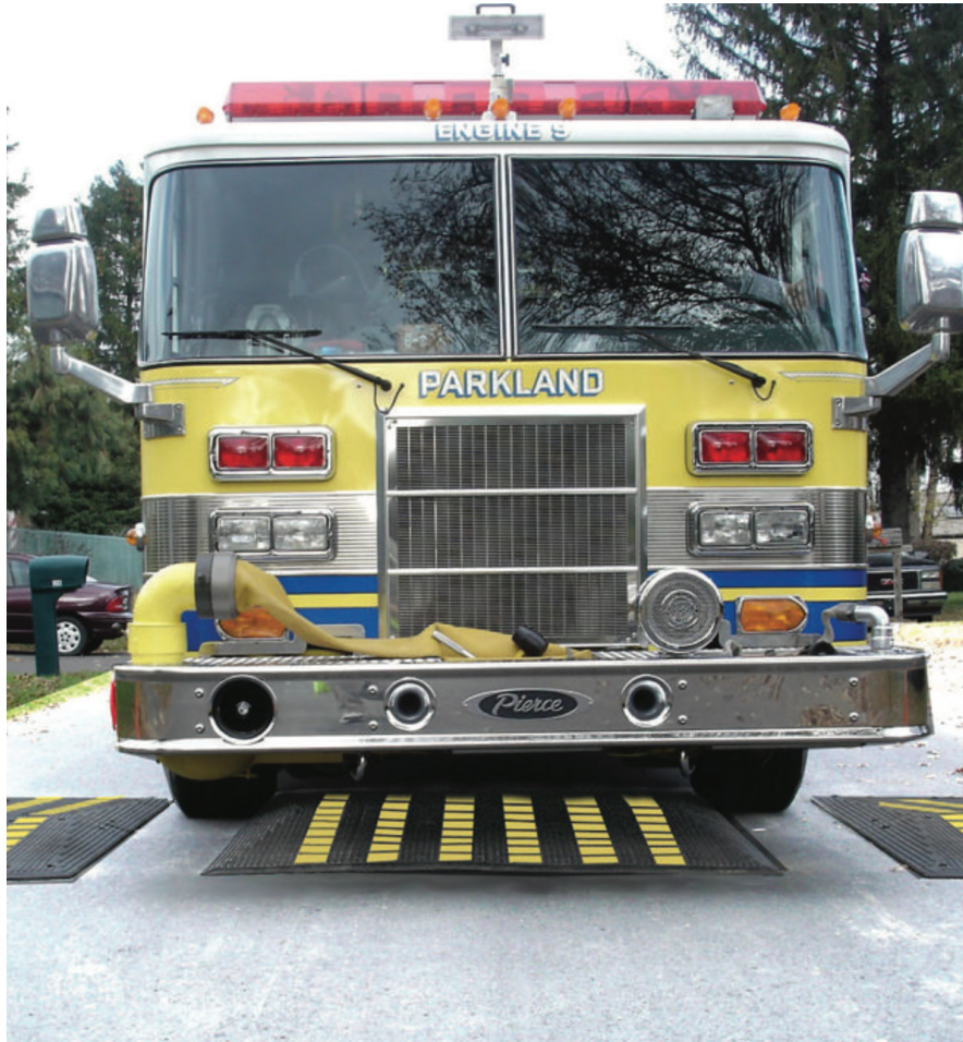
Speed cushions can be designed to provide traffic calming effects while not limiting access to emergency vehicles. Source: NACTO
