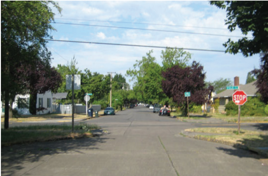
Neckdowns can shorten crossings for pedestrians at intersections along a greenway. Source: NACTO
