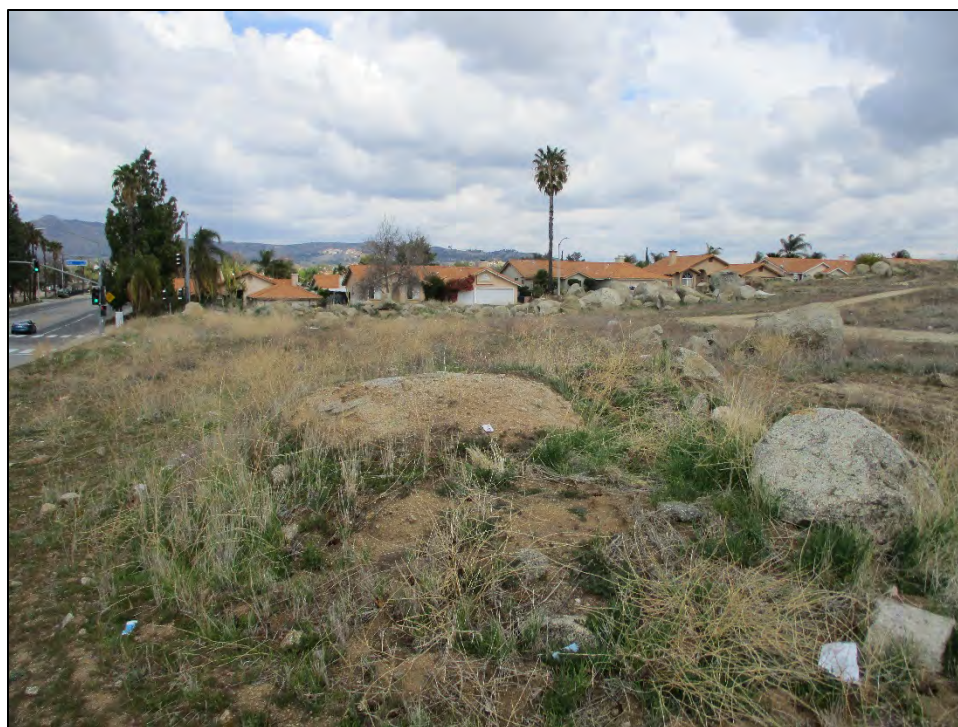
Figure 11. Exposed Cretaceous-age tonalite (Kt) at the surface along the south end of the Skylar Place tract in an area mapped as early Pleistocene-age very old alluvial fan deposits (Qvof). View facing to the north.
